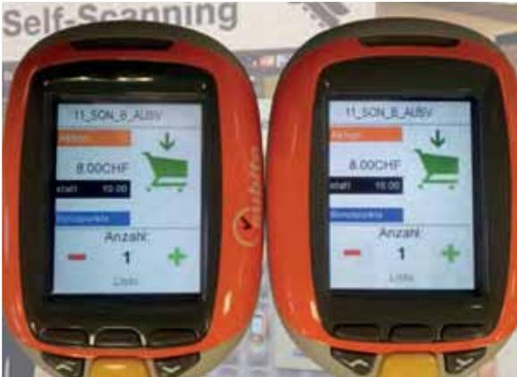
After the customer has scanned the product, the article is displayed on the colour display of the Motorola Solutions MC17.
